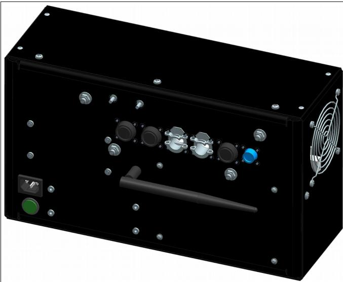
**Figure 6:** Replace plug in location highlighted in blue.
