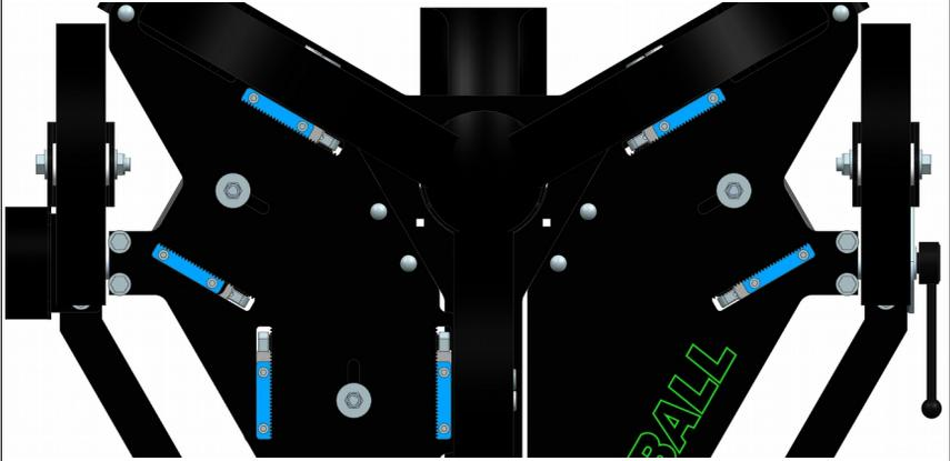
*Figure 4: Typical motor / wheel positioning for real softballs - motors are located at outermost position*
