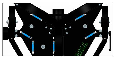
**Figure 3**: Typical motor / wheel positioning for real baseballs - motors are located one notch in from the center position
