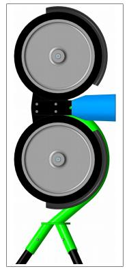
Figures 1 & 2: Install ball feeder tube as shown. Tube shown in blue.
