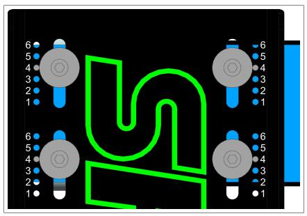
**Figure 3:** Top motor position numbering system. Motor sled locating pins shown in position 4 of 6. Motor sled shown in blue for clarity. Hole numbers are shown to illustrate numbering system only, and do not actually appear on machine.
