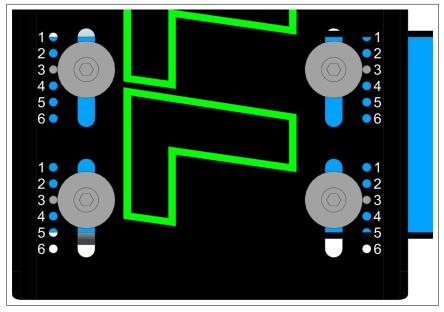
**Figure 4:** Bottom motor position numbering system. Motor sled locating pins shown in position 3 of 6. Motor sled shown in blue for clarity.
